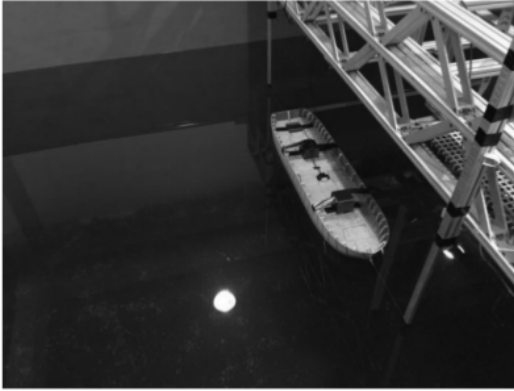
Figure 3: Setting model for a drift test in beam seas
